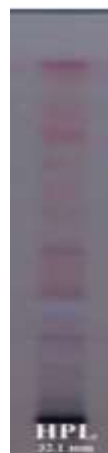
Plate 8: HPTLC profile of extract of H. pentandra with reference to Triterpenes after derivatization leaf
